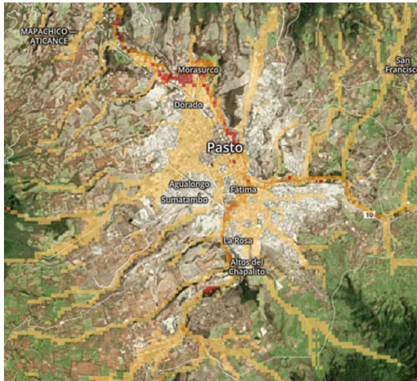
Figure 7. Pasto 100 year fluvial and pluvial flood map (Source: KatRisk with data set licenses by Willis Towers Watson)
